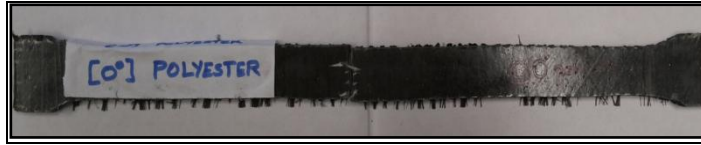
Fig 11 Carbon/polyester at [\pm 0^\circ] angle ply composite laminate specimen after tensile test
