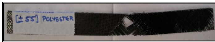
Fig 21 Carbon/polyester at [\pm 55^{\circ}] angle ply composite laminate specimen after tensile test
